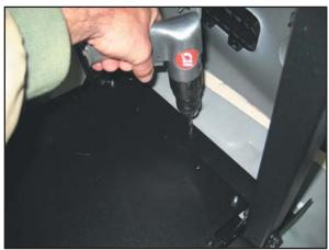
Bottom frame mount attaches to the trunk side floor. Drill three pilot holes with a 1/8" (.125") drill bit. \* Always check under floor before drilling \*
